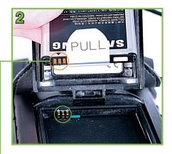
2) If replacing battery, use PULL tab to remove the battery. If receiving a new HMC Handheld, insert battery. Remember to turn the battery so that the battery contacts align with the Contact Position indicator mark (ORANGE Circle)
