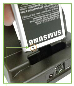
Insert a spare battery into the rear receptacle of the **HMC Handheld Dock**, with Contact Indicator (ORANGE Circle) pointing downwards to charge. This spare battery can be "hot swapped" when the external battery runs low, to extend the battery life of the HMC Handheld.
