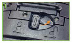
Slide the battery door hatch to the unlocked position (Right)
