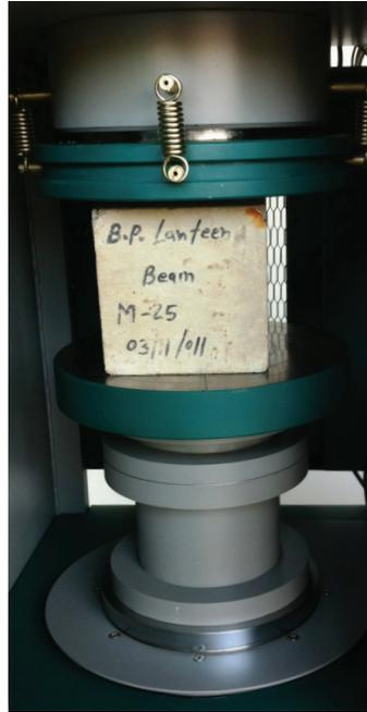
The installation of a simple manual valve system enables the flexural strength of concrete beams to be tested, up to 100kN (22,000lbf) maximum load.
