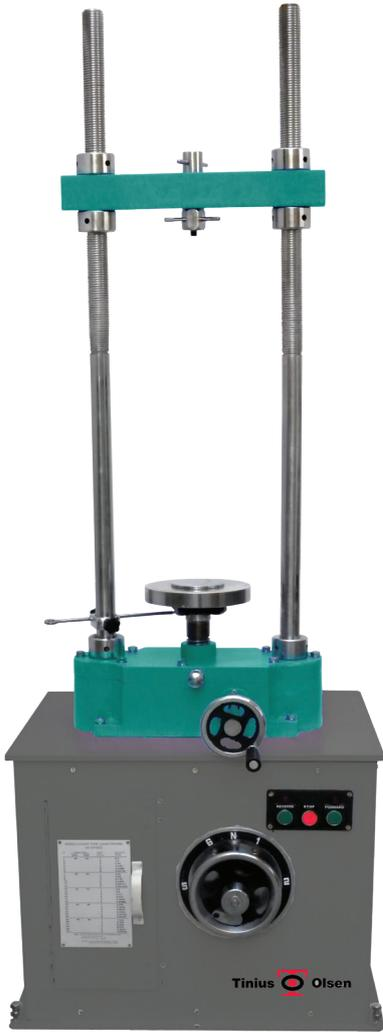
rock sample is cut to length and the ends are machined flat. The specimen is placed in a loading frame and, if required, heated to the desired test temperature. Axial load is continuously increased on the specimen until peak load and failure are obtained.
