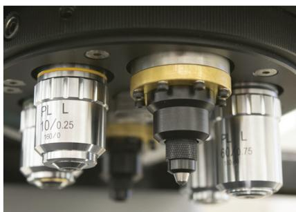
The turret can be configured with one or two indenter actuators, and combined with a maximum of four objectives. The second indenter can be added after installation.
