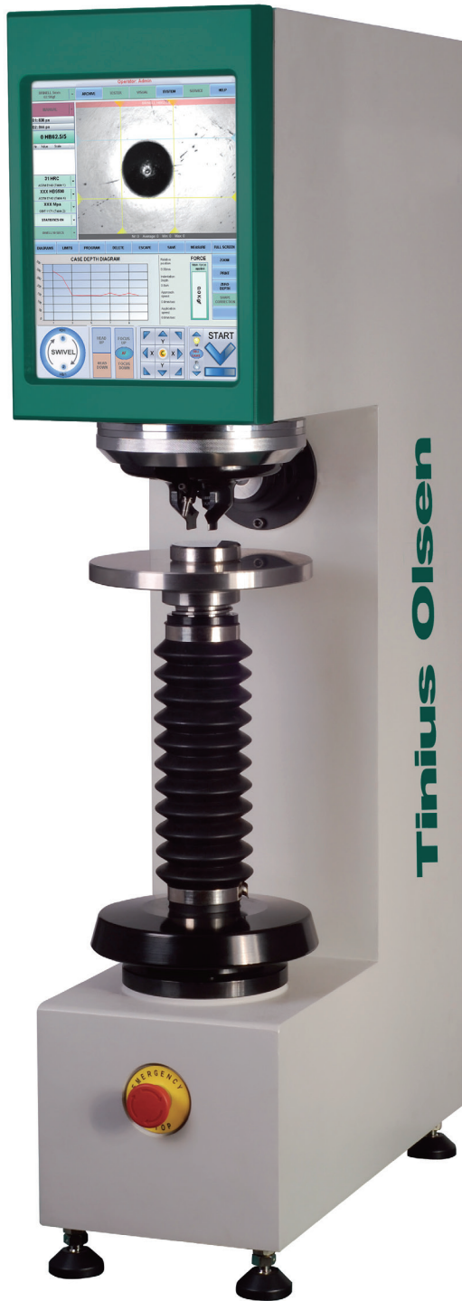
Model FH-10 Universal Hardness Tester with video indent measuring system
