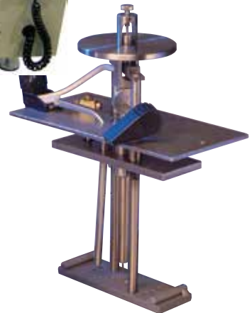
Fig 1. Model 603 HDTM shown with two test stations, one for deflection temperature and one for Vicat testing. The stations are raised for easy and rapid specimen insertion prior to a test and for specimen removal at the end of the test.
