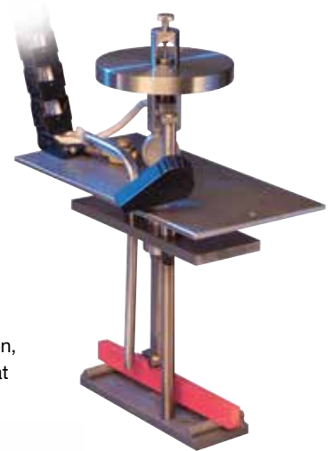
Fig 2. Model 303 HDTM shown with optional third test station, for deflection temperature and / or Vicat testing. Model here shown with three stations, gantry lowered, and optional cooling connections.
