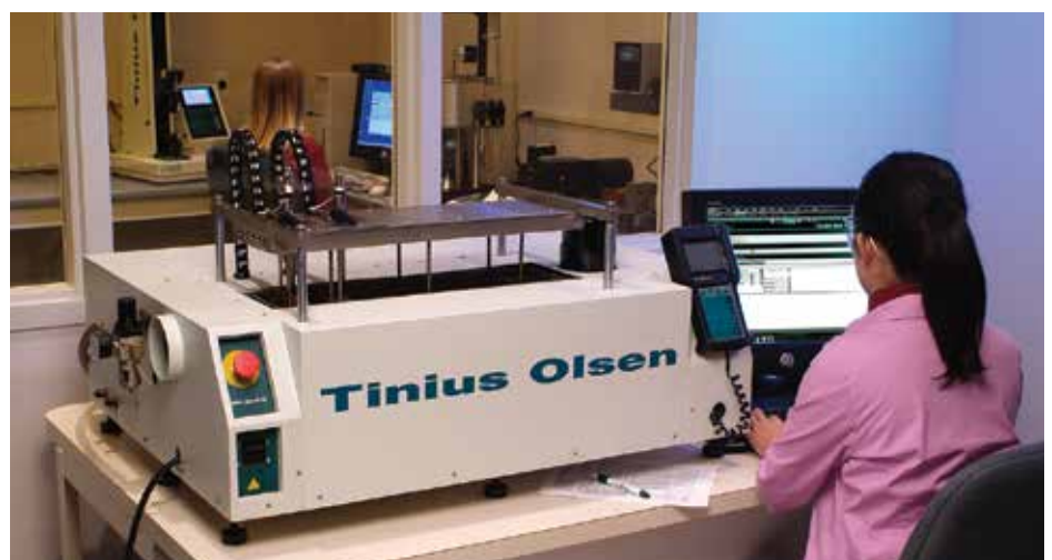
Fig 5. Both the Model 603 HDTM and 303 HDTM can be controlled by a PC.
