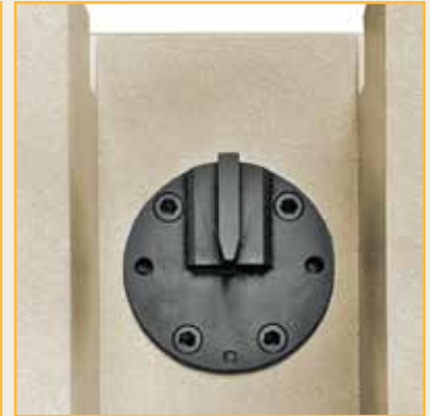
Charpy configuration. The specimen rests horizontally on the Charpy supports (obscured by the protective shrouds). Charpy centering tongs can be seen in front. To the right is an image of the striker.
