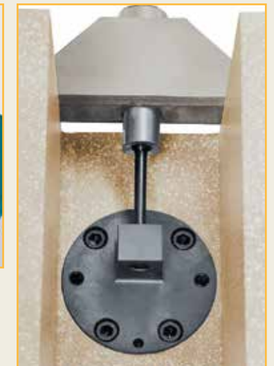
Tensile Impact configuration. The specimen is threaded into the "striker" and the holding bar at the rear of the pendulum head.
