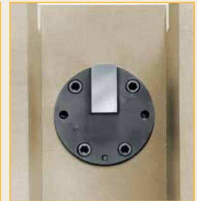
Izod configuration. The specimen is clamped in the vertical position at one end, using the front screw/vise. To the right is an image of the striker.
