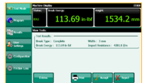
Touch screen display for machine and test set-up and display of results
