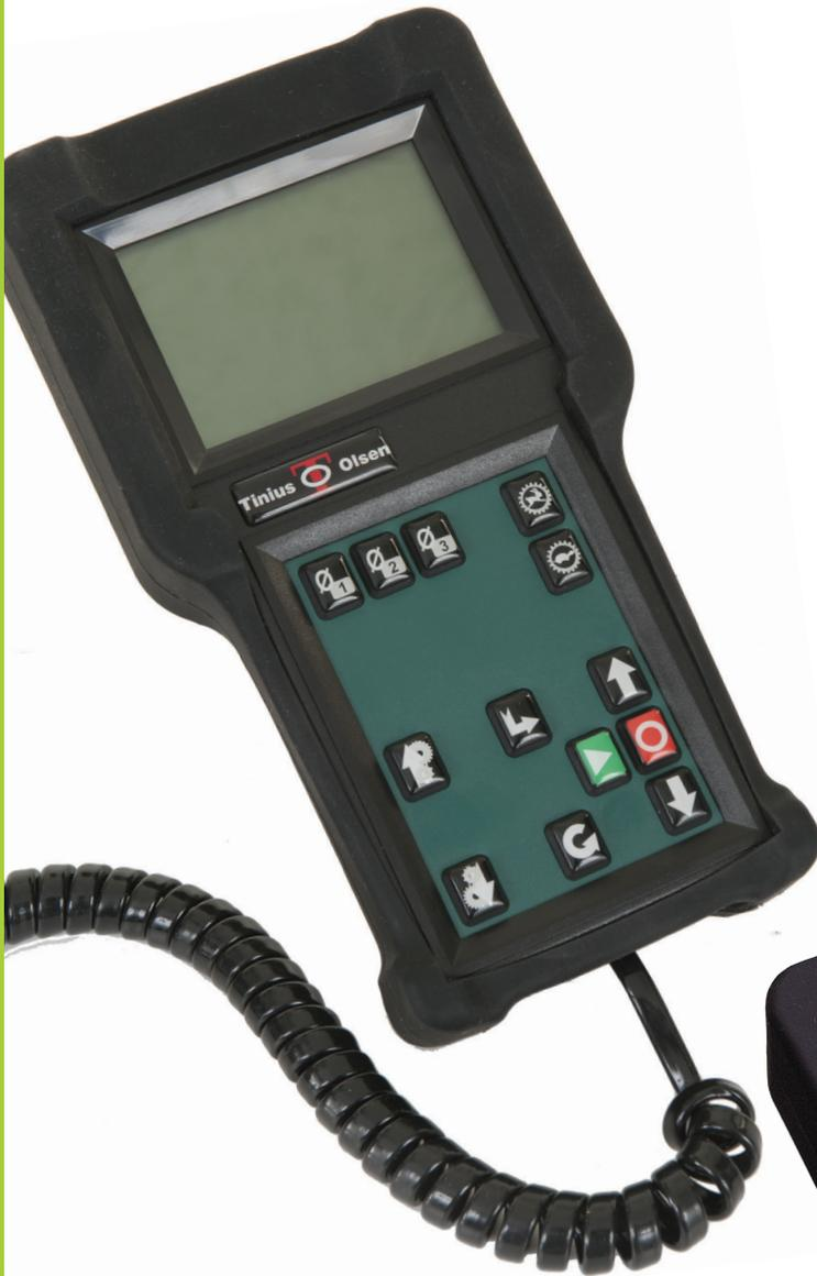
Familiar handheld controller that is tethered to the machine by an articulated arm. With its larger, tactile, sealed keypad, this controller is ideal for operators who use gloves to load and unload specimens and prefer a push button keypad. The controller can be used for basic operation of the tester and can initiate a test, but must be used with Horizon software.
