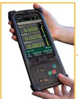
Wireless handheld interface which is connected to the machine by a Bluetooth link. This interface features an Android based operating platform and can be used to control the machine by itself or in conjunction with Tinius Olsen's Horizon software.
