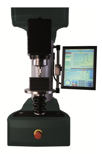
FH-011-0032 is a high speed Rockwell hardness tester designed to meet the needs of QC/QA engineers and technicians in a manufacturing environment. The FH-011 combines closed loop control and measurement technology with a colour touch screen user interface to achieve accuracy, repeatability and portability of test results whether used by single or multiple operators. Unbeatable GR & R results.
