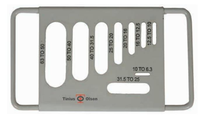
Aggregates that are flaky and/or elongated will often lower the workability of a concrete mix, and may also affect long term durability. In bituminous mixtures, flaky aggregates make for a harsh mix and may also crack and break up during compacting by rolling. The flakiness of aggregate is determined by measuring the thickness of individual particles. We offer both a thickness gauge and length gauge to check the flakiness index and elongation index of the aggregate respectively.
