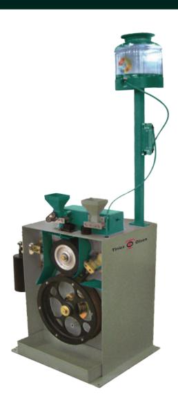
inius Olsen manufactures state-of-the-art Aggregate Polishing Machines. Specimens are manufactured in accurately machined and matched molds. They are then removed from the molds and located on the 'Road Wheel'.
