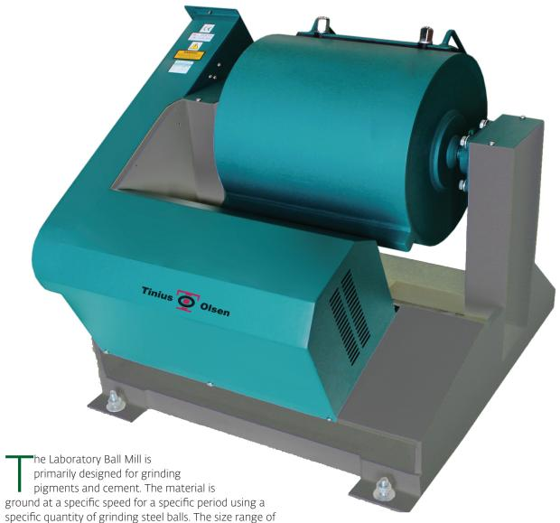
specific quantity of grinding steel balls. The size range of balls provided to support the tests is from 12.5 to 40mm. The size of ball varies with the requirement of the tests and complied standard. The Laboratory Ball Mill capacity also varies according to the application and ranges from 5-20kg.
