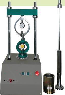
arshall Stability Test Equipment is used by highway departments, contractors, engineers, testing laboratories and other government agencies to test the stability of bituminous samples.
