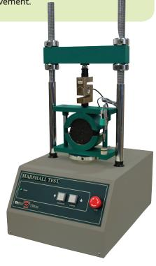
arshall Stability Test Equipment is used by highway departments, contractors, engineers, testing laboratories and other government agencies to test the stability of bituminous samples.
