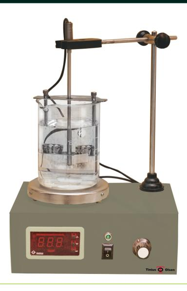
his equipment is used to determine the temperature at which a sample of bituminous material loaded by a 9.5mm diameter steel ball drops a specified distance when heated under specified conditions.
