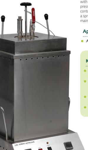
he Cement Autoclave is ideal for conducting accelerated soundness tests on cement and consists of a stainless steel pressure vessel with insulated outer shell. The temperature and pressure are measured by RTD probes and the system controlled by a PID controller, but the system has a spring-loaded pressure release safety valve to maintain safe operation.
