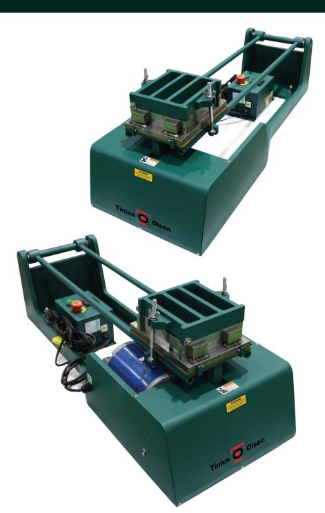
The Jolting Apparatus is used for making standard rectangular specimens measuring 40.1 x 40 x 160mm of Portland and Pozzolana cement mortar for determining transverse strength.
