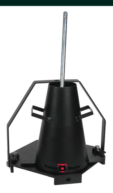
he Sheet Steel Slump Cone is filled with freshly mixed concrete and tamped with a tamping bar in four layers. The top of the concrete is levelled off with the top of the slump cone; the cone is lifted off the base and the slump of the sample is immediately measured.
