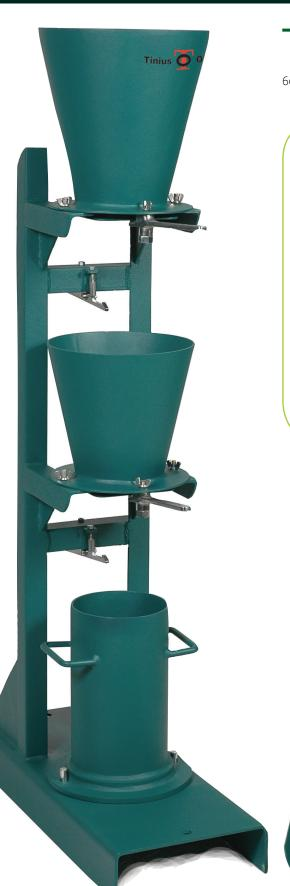
he Compaction Factor Apparatus consists of a hopper and receiver assembly: TO-345 tamping rod measuring 16mm diameter x 60cm long with a hopper and two trowels.
