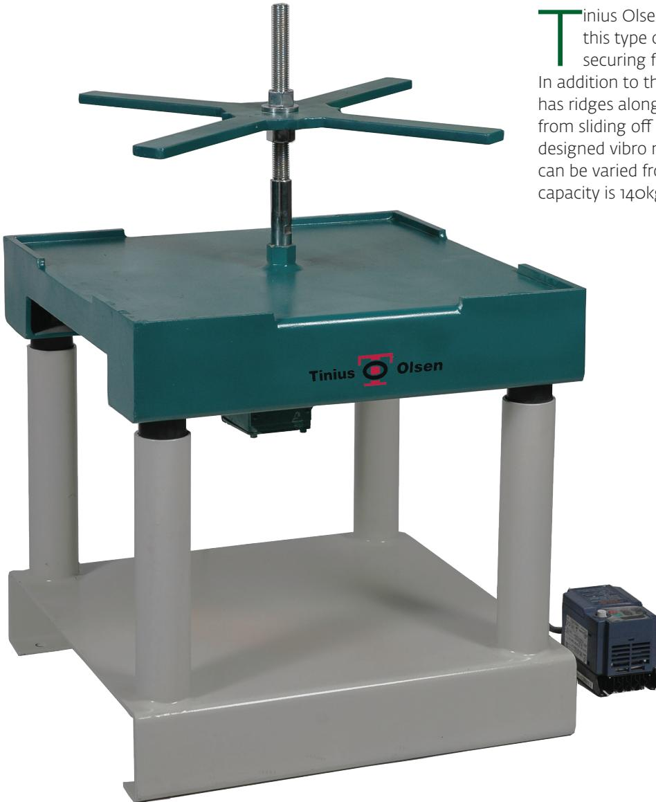
Tinius Olsen's Vibrating Table is ideal for this type of compaction and capable of securing four 150 mm cube molds at once. In addition to the securing clamp, the table has ridges along its edges to prevent molds from sliding off during operation. The specially designed vibro motor means vibration frequency can be varied from 60Hz to 43Hz. Maximum load capacity is 140kg.
