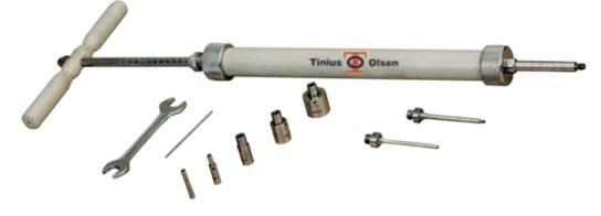
Compaction control in the field is exercised by determining the moisture content and dry density. Quick evaluation of this is done by developing curves in the laboratory, showing the relationship between moisture content versus dry density and penetration resistance, using Proctor Needles while conducting the Standard Compaction tests.
