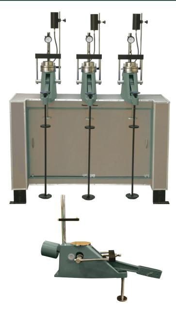
The Consolidation Apparatus consists of a fixed ring type of consolidometer cell for testing specimens of 60mm dia x 20mm thick, but a variety of specimen sizes from 50 to 100mm dia can also be tested. Additionally, the same loading unit can be used with optional floating ring consolidometer cells.
