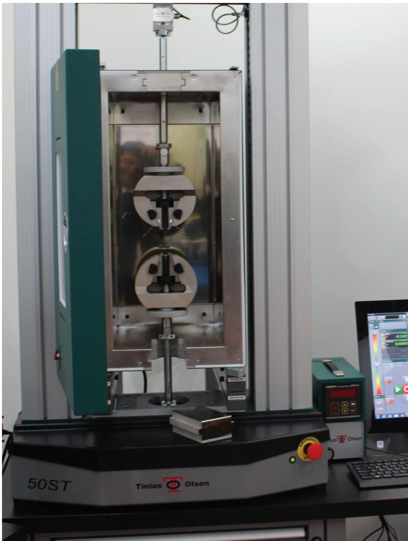
Suitable for most twin screw materials testing machines, the Tinius Olsen Environmental Chamber provides a means for performing physical tests within a temperature range of  $-70$ - $300^{\circ}\text{C}$  ( $-95$ - $570^{\circ}\text{F}$ ).
