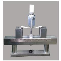
LVDT transducer kit and a mounting bracket also accompanies this flexural assembly. Graduated scale on main body of the unit allows accurate setting of support span.
