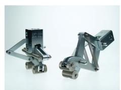
use two knurled rollers. The grip is particularly efficient for testing flexible dumbbell specimens. The centreline of the specimen remains constant in relation to the test machine, irrespective of the specimen thickness.
