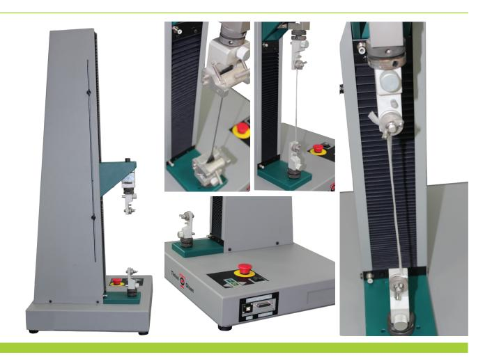
The model 5kL is an Electromechanical Materials Testing Machine. It is a robust design for use in a range of materials testing.
