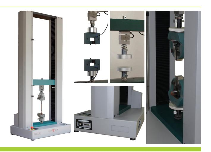
The model 10kL is an Electromechanical Materials Testing Machine. It is a robust design for use in a range of materials testing.
