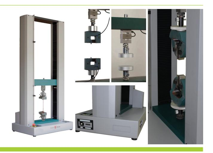
The model 50kL is an Electromechanical Materials Testing Machine. It is a robust design for use in a range of materials testing.
