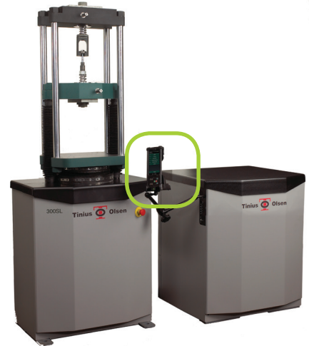
Typical 150kN (30,000lbf) SL with handheld controller.
