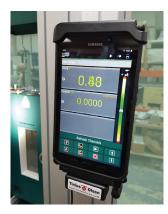
The Bluetooth connected interface features easy to operate tactile buttons and a high resolution touchscreen to set up and monitor tests where parameters and results are shown numerically. The interface also features an 8MP camera and has WiFi connectivity.
