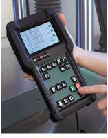
The tethered interface option features larger tactile feedback buttons to operate the testing frame; these are ideal for users who need to wear protective gloves while operating the machine. The display provides simple numerical display of individual channels used on the testing machine.
